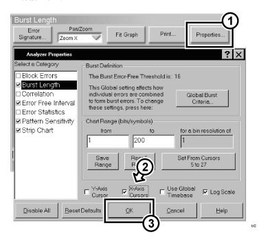
b Select Cursor x1 from the Pan/Zoom list. Touch and drag the cursor, or use the front panel knob to move the cursor to the desired position. Select Cursor x2 and repeat.
