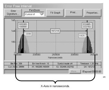
**8** Invert the time period between peaks to find the frequency of the interference.
