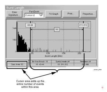
Histograms distinguish event occurrences by some metric. Cursor area measurements allow further quantifications of how many occurrences fall within some range of that metric. This is especially important when histogram entries may be shaped as a distribution of events, centered about some value, rather than one single, precise spike. Using the cursor area function, it is easy to "add-up" all the entries in a distribution surrounded by the cursors.
