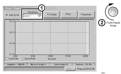
**b** Select **Pan Y** from the **Pan/Zoom** list. Touch the display and drag down, or turn the front panel knob counter-clockwise.
